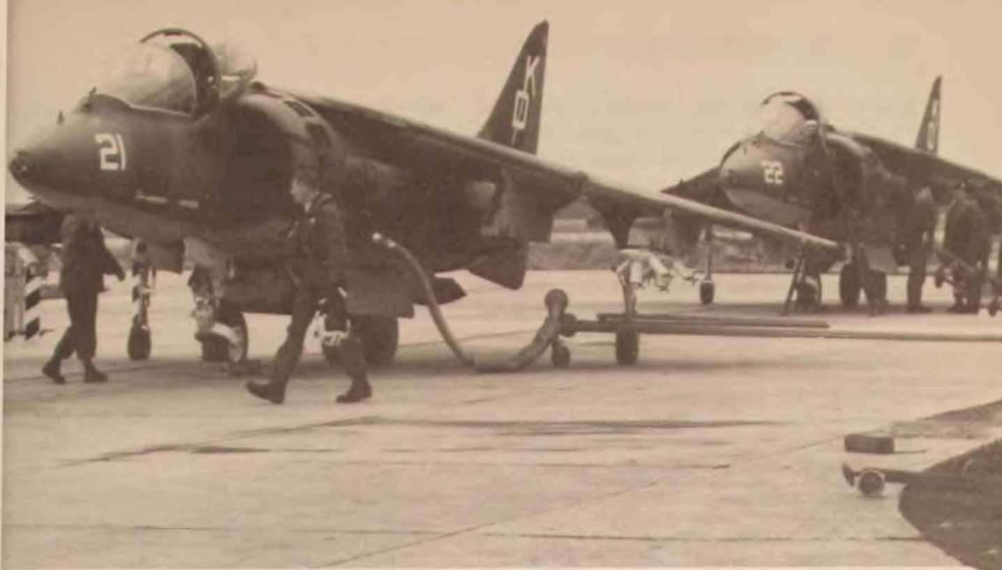
The inherent mobility of the V/STOL Harrier make it a natural candidate for the hide basing concept. From their secluded hides, the Harriers could remain operationally effective while presenting a multifaceted targeting problem to any aggressor.
